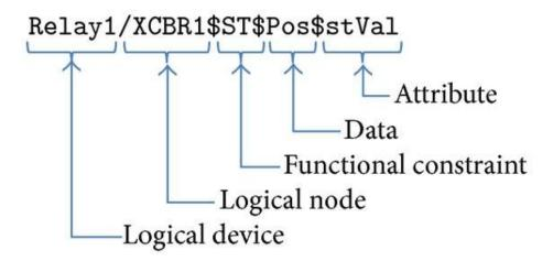
**LD - Logical Devices** - These are logical devices within this physical server, which work as function containers (Logical Nodes) or even as gateways between different LD LNs. Generally, IED internal names are used in the initial part of the name (prefixes) and suffixes that indicate the main function of the LD. Examples of suffixes are CTRL, MEAS, etc.
