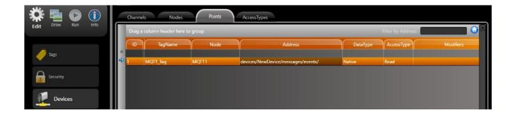
Once the device configuration is complete, go to *Run* > *Startup* and execute the project. Enable the Debug and Devices options by clicking on settings and selecting the corresponding boxes. Open the TraceWindow and monitor the communication exchange.
