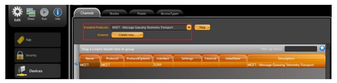
In Devices > Nodes, add a node for the newly created MQTT Channel. The primary station's configuration is made as follows:
