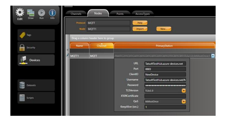
Finally, in **Devices > Points**, fill in the address information according to the syntax below:
