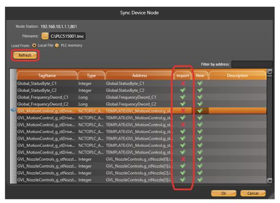
When you finish verifying and selecting the TwinCAT tags, click the Ok button to create the Tags, Templates, Device Channel, Node, and all Points.
