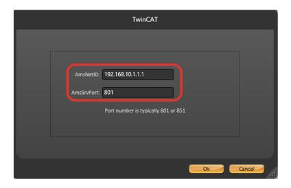
After adding the AMS Net ID and Port, the TwinCAT import dialog will appear. This dialog contains two options to load the imported TwinCAT tags; Local File or PLC Memory. For the Local File, we need to configure which file you want to import. To configure it, you must use the Filename field and select the file name. TMC, TPY, and XML files are supported.
