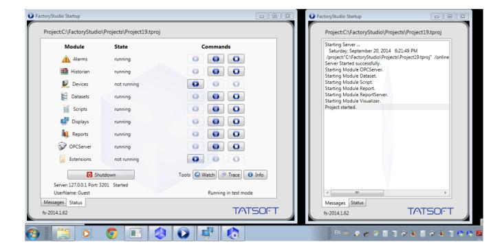
The main role of the TStartup.exe is to run the TSERVER.exe with the right set of parameters. The TServer application will load the project and the real-time tags. It is the main process that will allow the other modules from the same computer or remote computers to exchange real time data.
