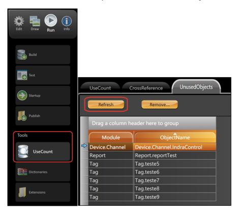
Any object that is found is an unused object. Select the object that you want to remove, and click "remove...". You can select multiples objects remove, or
