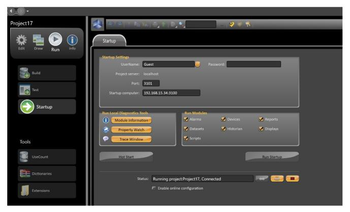
Hit the **Run Startup** button, and the project should start running on the Raspberry pi.
