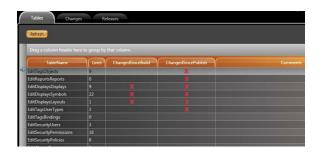
FactoryStudio tracks changes for every aspect of a project configuration. Whenever a table is created, its name will be displayed in this page. An "X" sign at "ChangedSinceBuild" and "ChangedSincePublish" columns will indicate if there were any changes, as shown in the image on the right.
