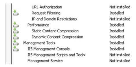
You can go back to the Compression module for your site and ensure Dynamic Compression is checked. At this point, Dynamic Compression should be set up, but you must be specific about what MimeTypes will be compressed.
