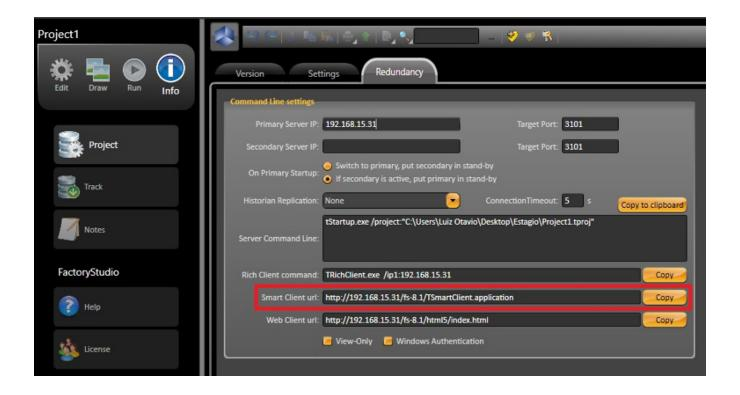
After setting the configurations, double-click on the shortcut file and keep it running. You should see a window open with a message saying the application is waiting for the *TServer* to run. Once the project is executed, the *TSmartClient* will open automatically.
