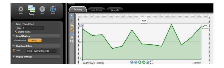
In runtime, the elements can be maximized by clicking on the button indicated by the (1) below or resized by dragging the button indicated by the (2) below.
