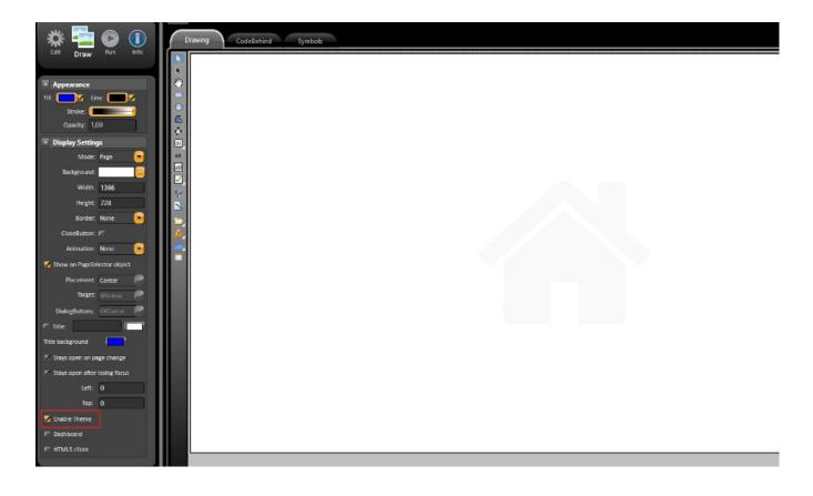
Individual components will have an Enable/Disable checkbox in the left panel settings.
