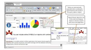
**FactoryStudio** includes a user-friendly, simple report layout editor integrated within the engineering workspace. The rich text format uses underlying XAML flow document technology from WPF that enables the inclusion of graphics and flexible formatting.
